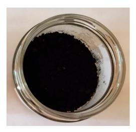
Figure 4. A sample of char powder produced by the PDG technology.
